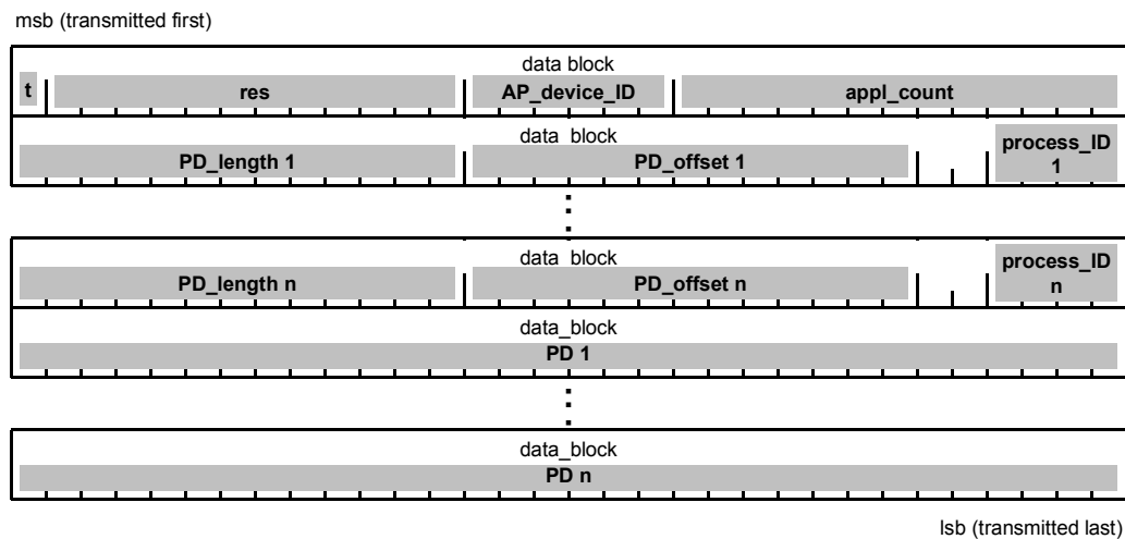
Figure 6.1 – Process Data APDU Structure
